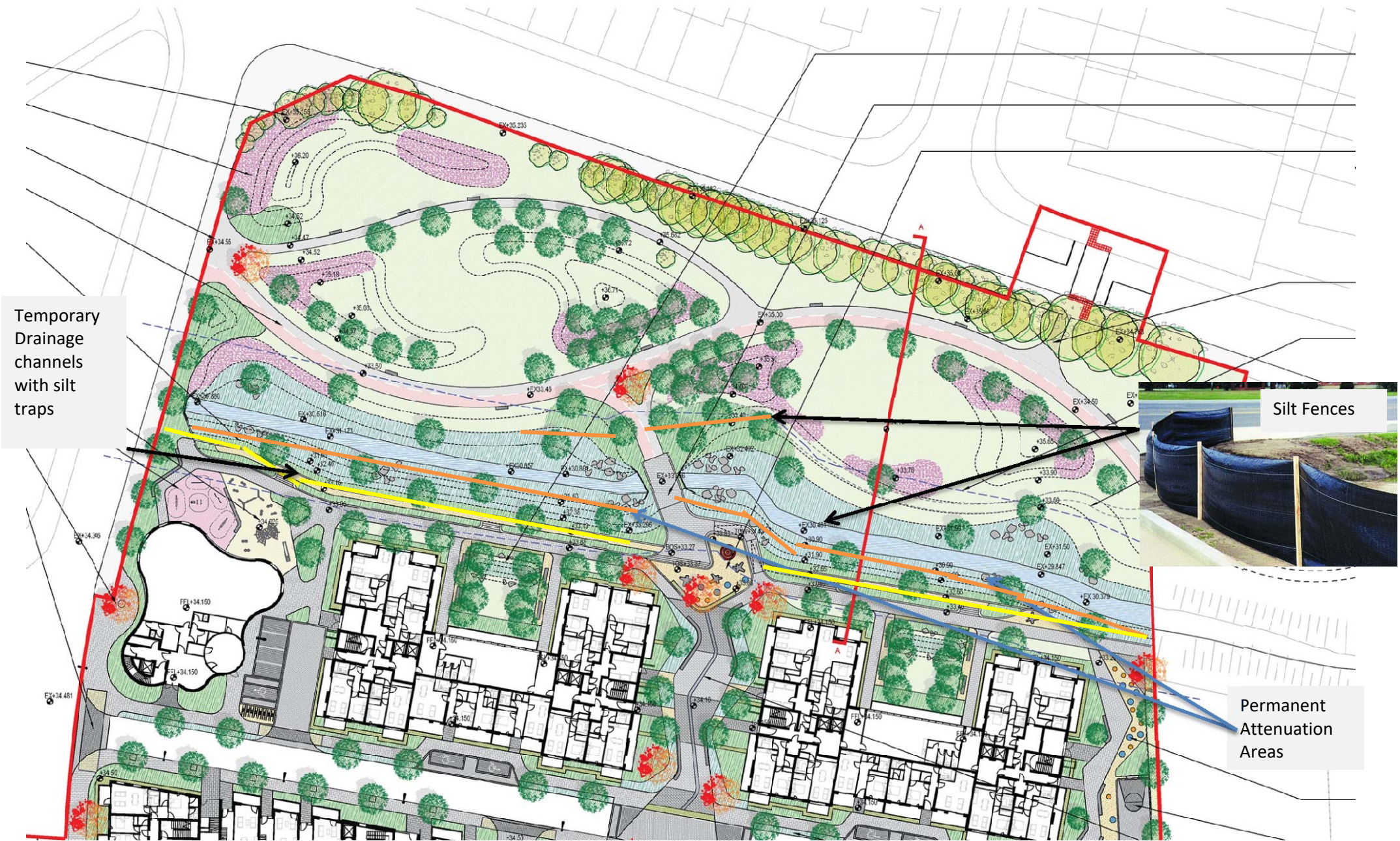
Figure 7. Mitigation measures to protect the Santry River
